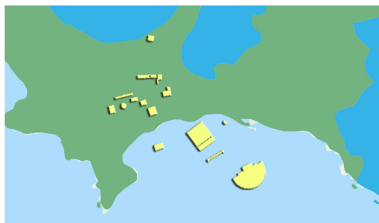
Figure 16. Geological map of Epidauros temple area (redrawn data from IGME). The location of the temple, shown in yellow, is placed in an area of intense geological change -a conductivity discontinuity- between glaucophane lawsonite epidote metamorphic rocks (shown in green), marble (shown in dark blue) and gypsum rocks (in light blue).
