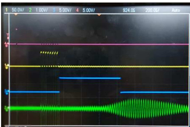
Figure 3. The different signals emitted and received by the HC-SR04 sensor observed on the oscilloscope. The pink curve represents the Trigger, the yellow curve the pulses emitted at 40kHz, the blue curve the Echo and the green.
